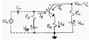
Design an amplifier with a peak amplification of  $|V_{out} \setminus V_{in}| = 20$ .
